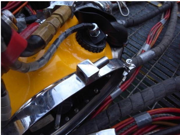
Helmet sealed pull pin slot after failure
