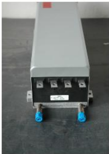
Image 2: new CCU (DC output)
